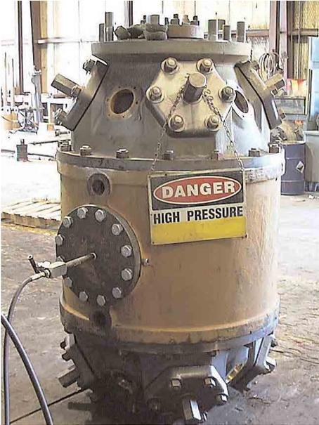
Compressor cylinder being hydrostatically tested at 1.5 times the maximum working pressure
