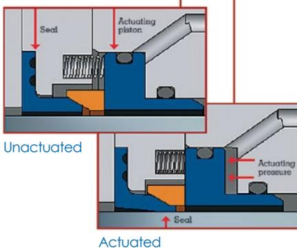
piston rod. The flexible polymer seal conforms to the rod circumference, locking in high-pressure gas.
