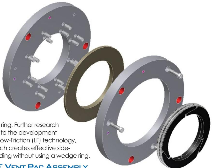
the ring. Further research led to the development of Low-Friction (LF) technology, which creates effective side-loading without using a wedge ring.
