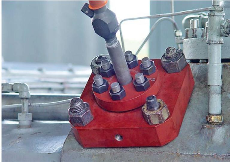
*Cook Indicator Ports access pressure through the center of a compressor valve and retain pressure with O-ring seals. This illustration shows an Indicator Port with an HSR high-strength restraint, which secures the valve using outside cap screws.*
