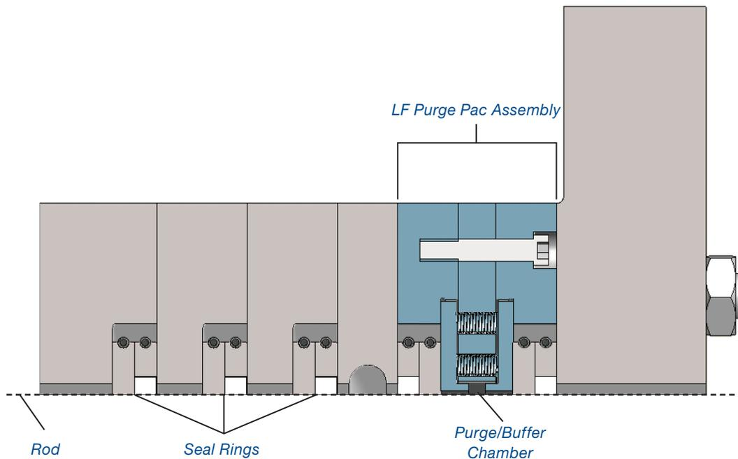
*LF Purge Pac assemblies are designed to fit most packing cases*
