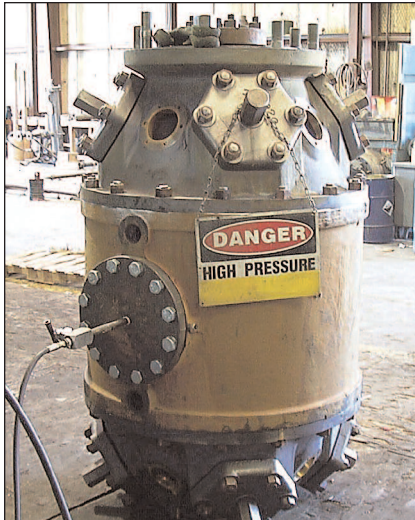
Compressor cylinder being hydrostatic tested at 1½ the maximum working pressure
