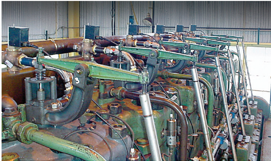
Integral engine equipped with Windrock AutoBalance system (above)
