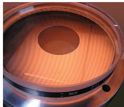
Optical comparator checks flatness of critical surfaces
